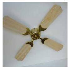
This is a 42" four-blade ceiling fan with tan or white painted wood blades and a bright brass housing. The 3-speed reversible motor is controlled by infrared remote control and draws 1.2 amps (on 12V models) at high speed, draws 0.75 amp at medium speed and draws 0.5 amps at low speed. This fan is designed for surface mounting on a flat ceiling. An 8" swivel pendant mount for pitched ceilings is available as an option. They are available for 12- or 24-volt DC operation. CSA/UL approved.
